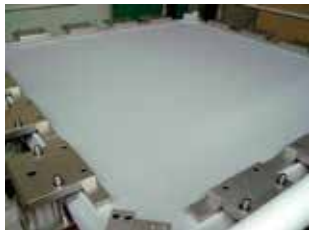
Fabric stretched to preset tension
