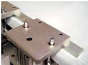
Automatic clamps grip mesh
